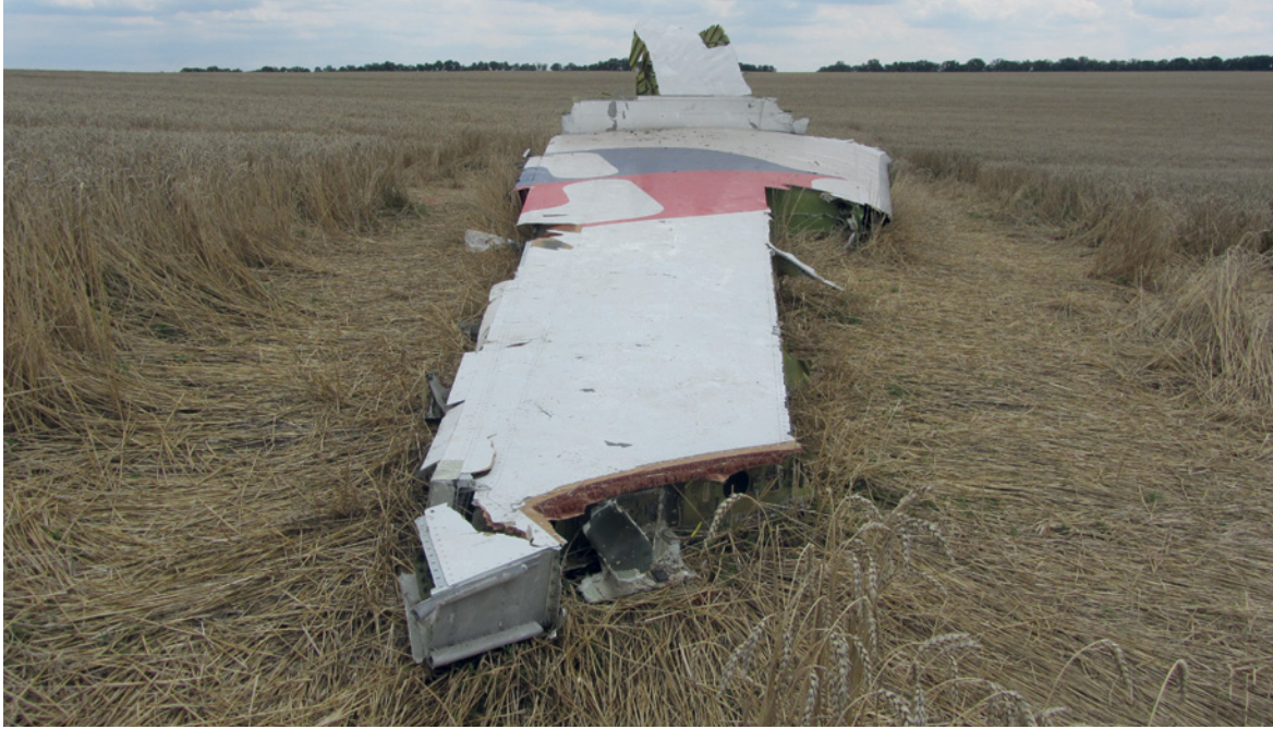
Figure 12: Vertical tail. (Source: DCA)
