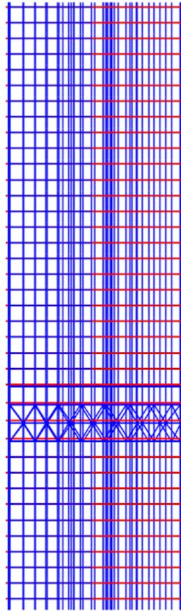
Figure 2.21 SAP2000 model for Floor 12 to Floor 47.
