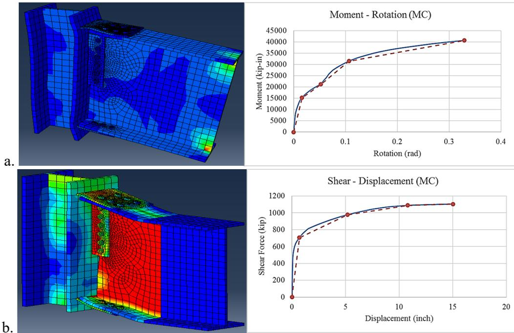
Figure 2.52 Moment connection (MC): a. moment-rotation, b. shear-displacement.
