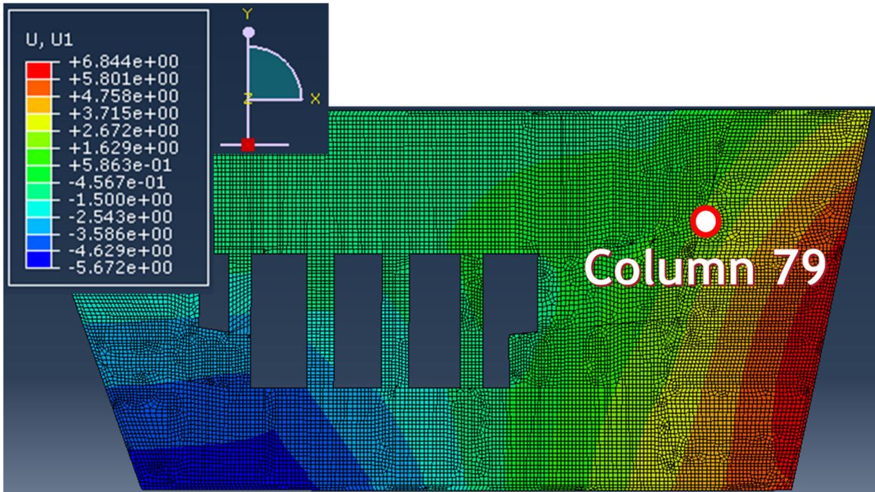
Figure 2.61 Movement in  $x$ -direction at Floor 13.
