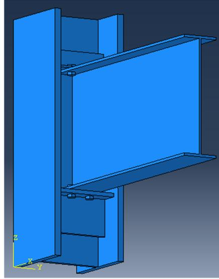
Figure 2.42 Seated top plate connection sample ABAQUS model.
