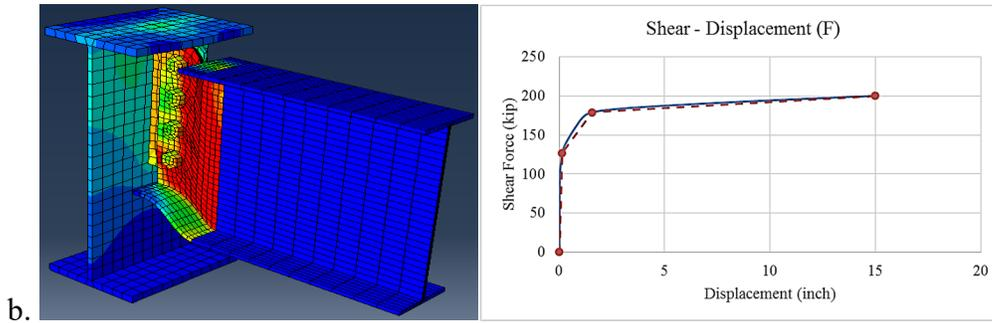
Figure 2.46 Fin connection (F): a. moment-rotation, b. shear-displacement.
