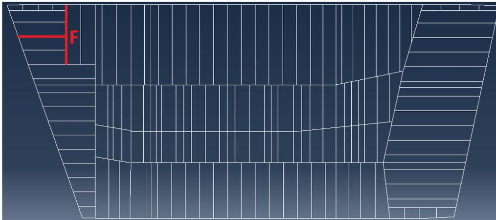
Figure 2.37 The location for a Type “F” Connector
