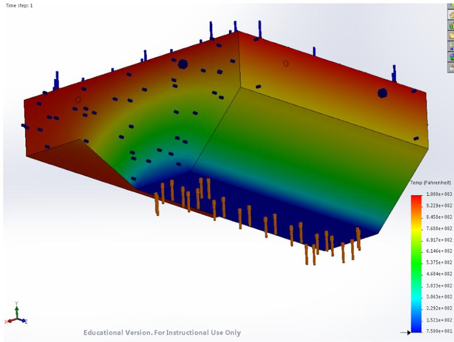
Figure 2.9 Temperature distribution of the unit floor slab.
