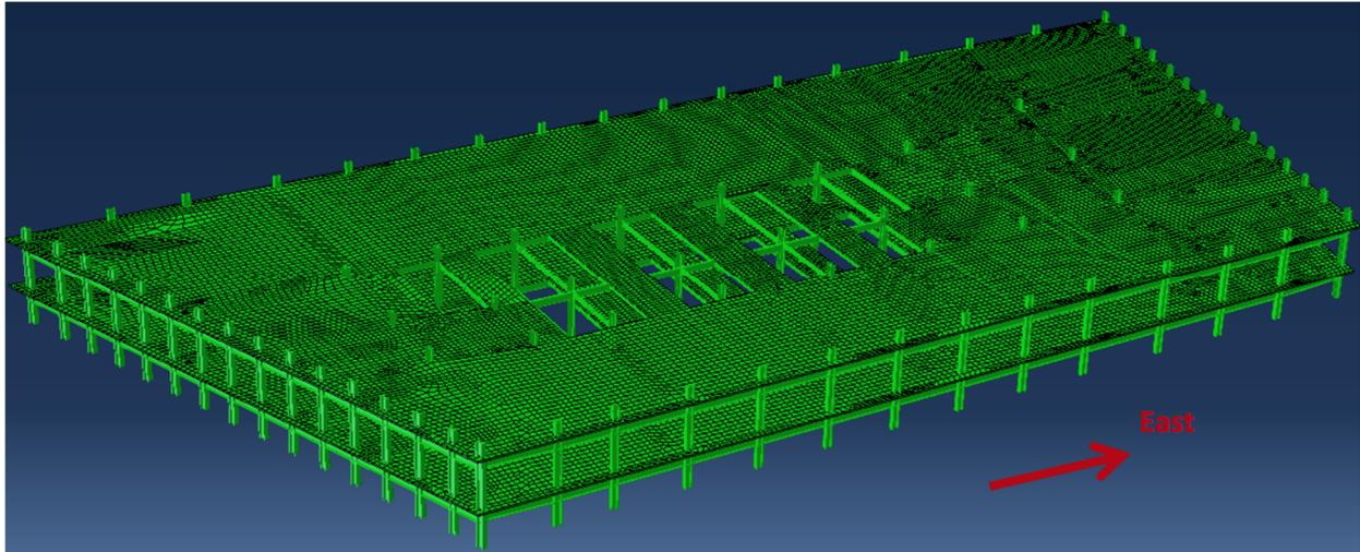
Figure 2.59 ABAQUS Model for Floors 12 and 13.
