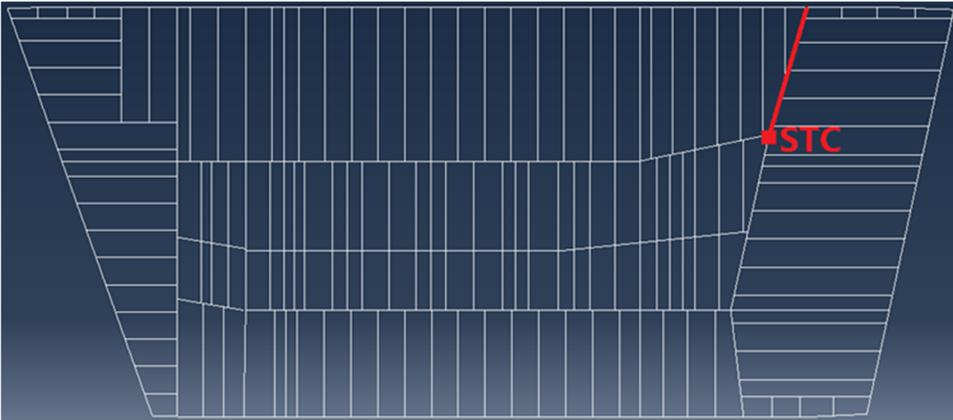
Figure 2.38 c. Nonlinear spring in WTC 7 modeling
