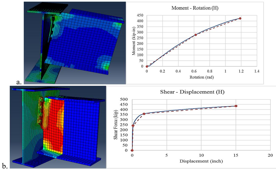
Figure 2.47 Header connection (H): a. moment-rotation, b. shear-displacement.
