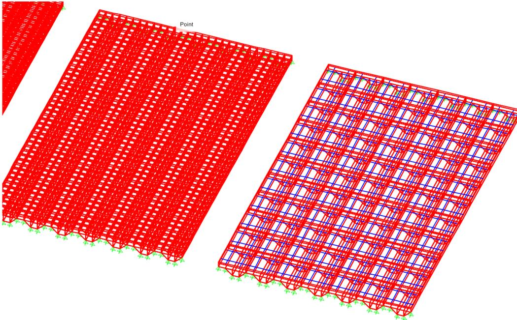
Figure 2.27 Models of floor slabs with different meshing.
