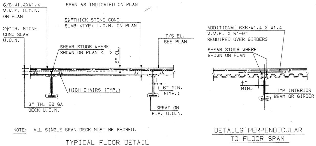
Figure 2.24 Typical floor detail of WTC 7.
