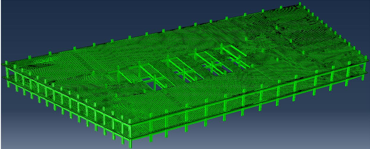
Figure 2.30 Floor 12 and 13 ABAQUS model.
