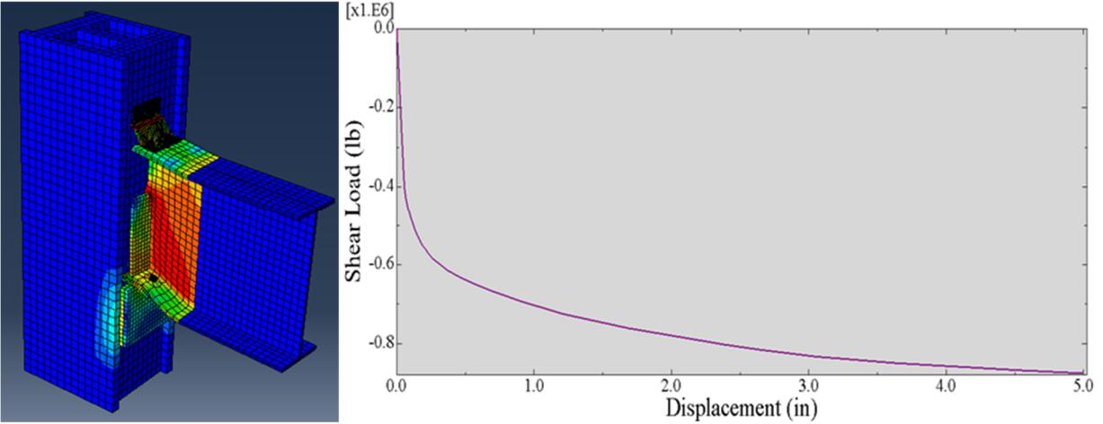
Figure 2.38 a. Connections modeling and shear-displacement nonlinear curve
